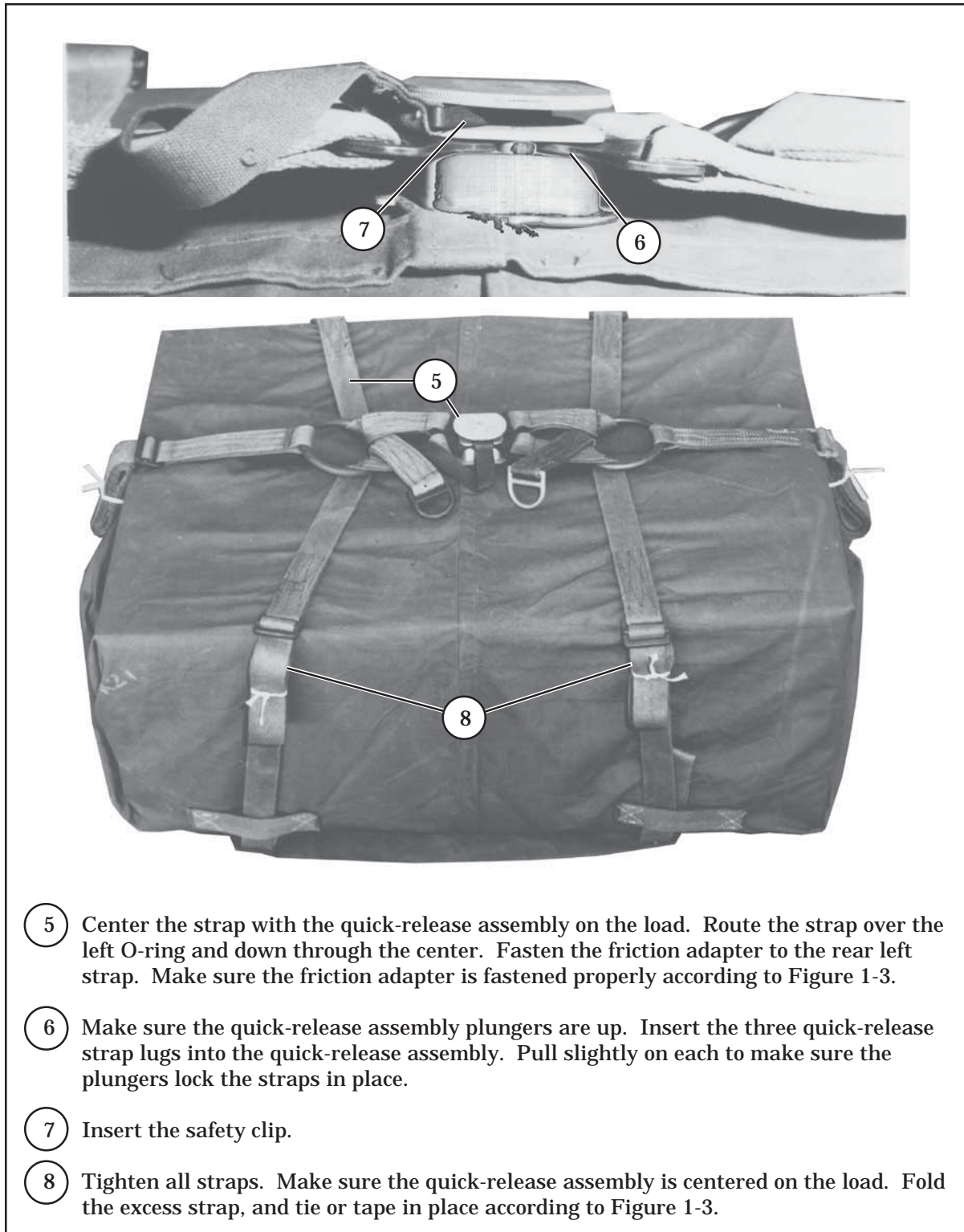
Figure 6-2. Container Rigged (Continued)
